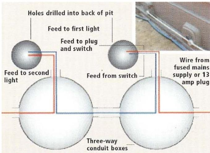
**7** Route the wires for switch, plug socket and lights. Use one conduit box behind the light switch and plug, and one each for the four lights. Use conduit (tube to protect wiring) for the wires between boxes (see inset). The feed from the switch to the first light goes into a connector. From here power is fed to the light and a live feed taken to the next light.
